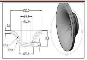
Fig: 1. Selected Component with Dimensions
