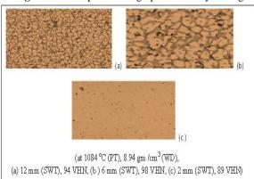
Fig: 13. Surface photomicrograph of Cu alloy casting
