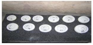
Fig: 4. Ready Shells for Pouring
