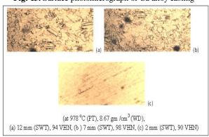
Fig: 14. Surface photomicrograph of brass alloy casting
