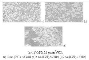
Fig: 11. Surface photomicrograph of Zn alloy casting
