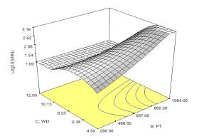
**Fig: 9.** Effects of PT and WD on Vickers Hardness Number
