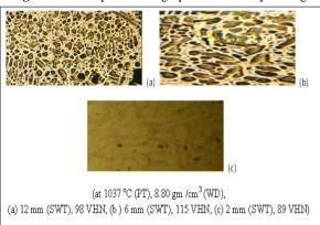
Fig: 15. Surface photomicrograph of bronze alloy casting
