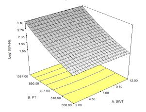
Fig: 7. Effects of SWT and PT on Vickers Hardness Number
