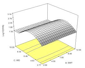
**Fig: 8.** Effects of SWT and WD on Vickers Hardness Number
